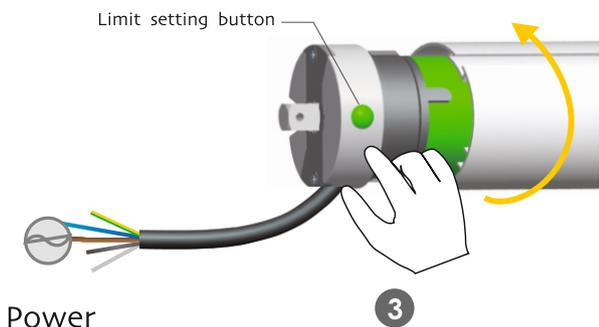
Release the setting button in the limit head namely confirm reverse limit position
