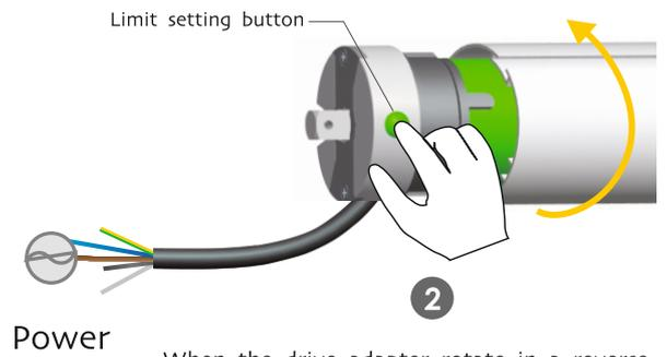
When the drive adapter rotate in a reverse direction or stop (the brown wire and blue wire connect with power), press the setting button in the limit head, the motor will rotate in a reverse direction
