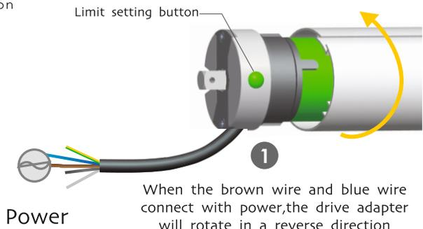
When the brown wire and blue wire connect with power, the drive adapter will rotate in a reverse direction
