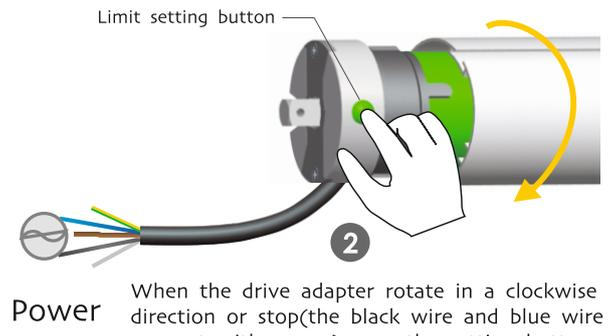
When the drive adapter rotate in a clockwise direction or stop (the black wire and blue wire connect with power), press the setting button in the limit head, the motor will rotate in a clockwise direction
