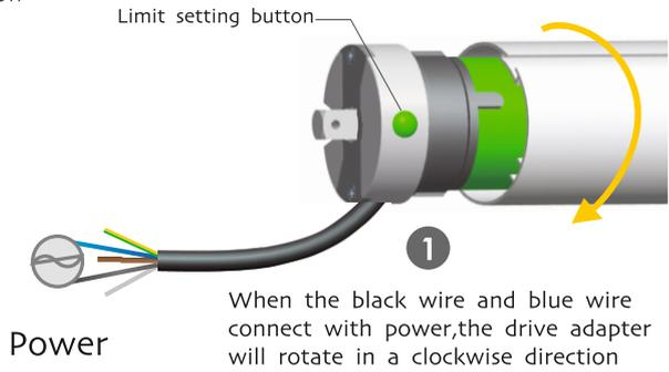
When the black wire and blue wire connect with power, the drive adapter will rotate in a clockwise direction
