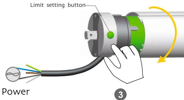
Release the setting button in the limit head namely confirm clockwise limit position
